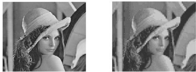
Fig. 3. Standard Image -Lena_gray.tif compressed by KSOFM neural network. (left) -Original image, (right) - decompressed image
